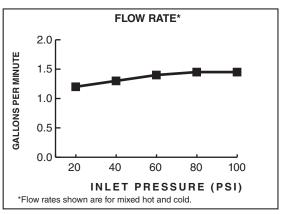
1.5gpm/5.7 L/min. FLOW RATE
