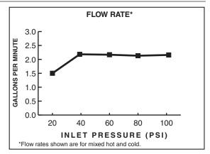
2.2gpm/8.3L/min. FLOW RATE
