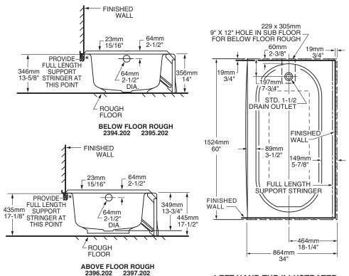
\*PLUMBER NOTE: PROVIDE FULL LENGTH SUPPORT STRINGER AT THIS POINT LEFT HAND TUB ILLUSTRATED RIGHT HAND TUB IS REVERSED
