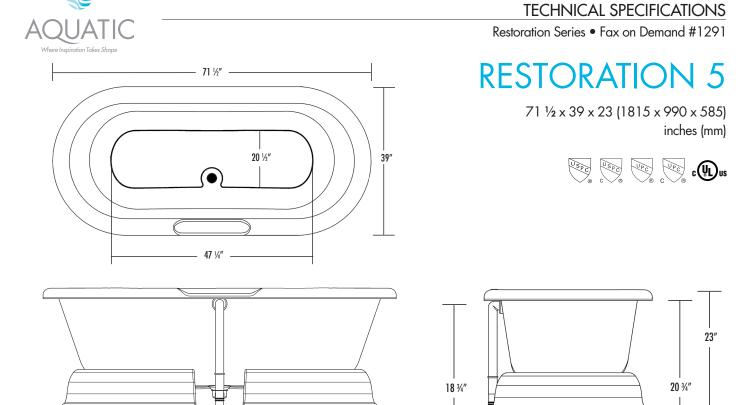
FEATURES Ibs (kg) Dimensional Tolerance ± 3/8". Dimensions needed for site preparation should be measured from the unit. Aquatic assumes no responsibility for preparatory work.
