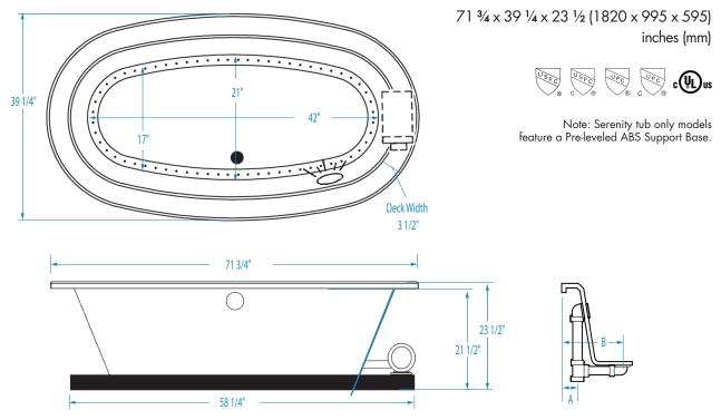
FEATURES lbs (kg) Dimensional Tolerance ± 3/8". Dimensions needed for site preparation should be measured from the unit. Aquatic assumes no responsibility for preparatory work.
