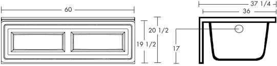
FEATURES Ibs (kg) Dimensional Tolerance  $\pm$  3/8". Dimensions needed for site preparation should be measured from the unit. Aquatic assumes no responsibility for preparatory work.
