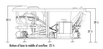
FEATURES lbs (kg) Dimensional Tolerance ± 3/8". Dimensions needed for site preparation should be measured from the unit. Aquatic assumes no responsibility for preparatory work.
