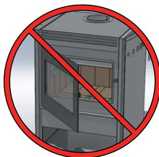
Never burn the appliance with the loading door open. Leaving the door cracked open may damage the combustor.
