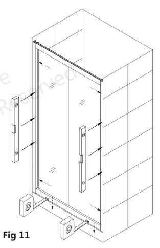
**12.** From inside of the shower, mark the screw holes onto the wall through the pre-drilled holes in flanges of the **Wall Profiles (#01)**.
