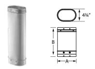
Use to reline masonry chimney with 0/0 clearance. Available in oval 6" and 8" diameters; 12", 24", 36", and 48" lengths. Factory-insulated. Built-in, pre-drilled fittings for riveting joints. 304 stainless steel inner and aluminized steel outer. Note: to calculate the installed length of 5", 6", and 8" DuraLiner pipe subtract 1 ½" from each joint overlap of liner pipe sections.
