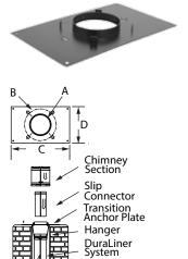
Use with Slip Connector and Hanger in chimney restoration to connect DuraLiner pipe to DuraTech, DuraPlus, or DuraPlus HTC Chimney. Painted black. Pricing for Transition Anchor Plates are listed under DuraTech, DuraPlus, and DuraPlus HTC.
