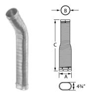
Use through damper and smoke shelf area. Use to connect from oval stove outlet to round DuraLiner. Use with DuraLiner Insulation Kit (ProMesh and ProFoil), where flex extends into clay liner, for zero-clearance applications. Built from 1-ply construction, .005" 304 stainless steel.
