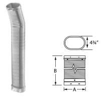
Use through damper and smoke shelf area. Use with DuraLiner Insulation Kit (ProMesh and ProFoil), where flex extends into clay liner, for zero-clearance applications. Built from 1-ply construction, .005" 304 stainless steel.
