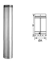
Use to reline masonry chimney with 0/0 clearance. Available in round 6" and 8" diameters in 12", 24", 36", and 48" lengths. Factory-insulated. Built-in, pre-drilled fittings for riveting joints. 304 stainless steel inner and aluminized steel outer. Note: to calculate the installed length of 5", 6", and 8" DuraLiner pipe subtract 1 ½" from each joint overlap of liner pipe sections.
