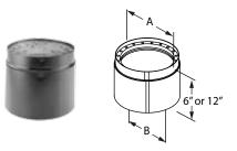
Use to add length to DVL pipe. 6" pipe adds 2" - 5" of length, 12" pipe adds 2" - 11" of length, when used with rigid sections of pipe. 12" section can be ovalized for oval-to-round appliance connector.
