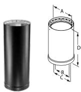
Designed for installation with minimum clearance to combustibles (6" to walls, 8" from top of horizontal run to ceiling). Available in 6", 7", and 8" diameters. Subtract <sup>3</sup>/<sub>4</sub>" for installed length. Constructed with a stainless steel inner wall.
