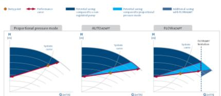
Proportional pressure mode is used in circulating systems. The pump continuously adapts its performance to the varying flow demand. The AUTOAWET function continuously adjusts the proportional pressere curve and automatically sets a more efficient one, without compromising confort demands. With this factory setting, in 80% of the installations no manual adjustments are needed.
