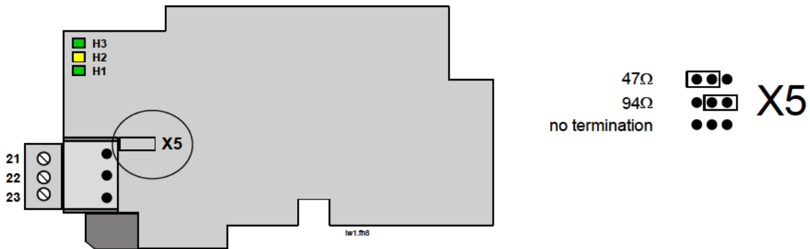
Figure 11. Using jumper X5 to set the bus termination
