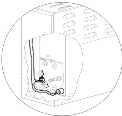
All CT models have Express Steam standard. Express Steam is equipped with a low power heating element and thermostat to keep the water in the tank warm enough to bring up steam quicker. All Express Steam components and wiring are installed at the factory. No additional wiring or plumbing is required by installers.
