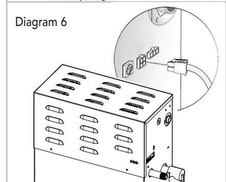
**IMPORTANT NOTE:** The control cables should be run in dedicated 1" conduit to facilitate installation and service.
