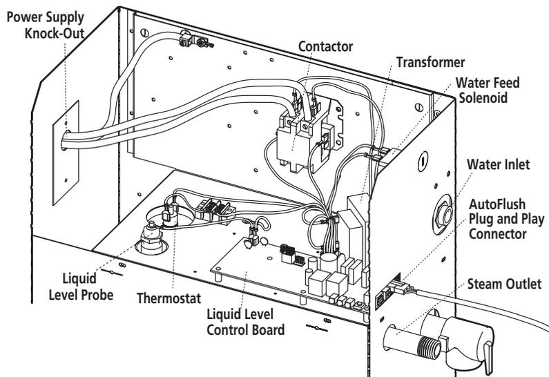
main voltage on the load side of the contactor when it is engaged.
