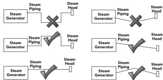
**⚠ WARNING** Failure to pitch the steam piping as required for condensate to drain, may cause condensate to block the flow of steam. Blocking the steam flow may cause steam pressure to discharge boiling water through the steamhead, resulting in a scalding hazard. Blocking the flow of steam may cause steam to discharge through the safety valve, resulting in a scalding hazard.
