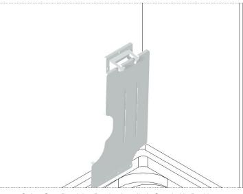
Safety Seat Retaining Bracket Installed. Seat In Up Position.
