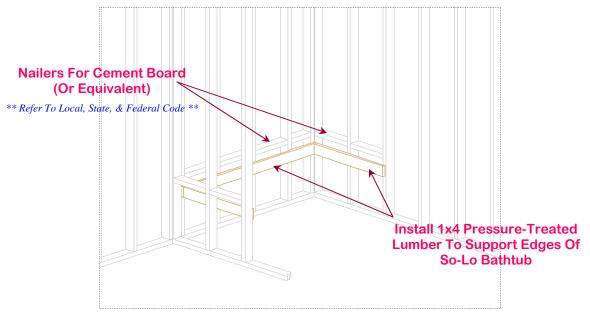
Safety Bath So-Lo Support Framing And Cement Board Nailers
