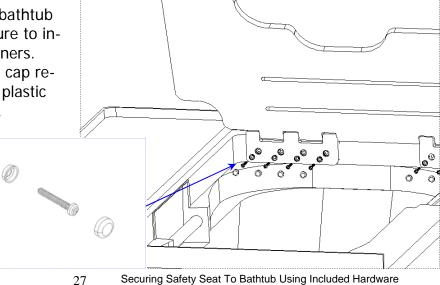
Securing Safety Seat To Bathtub Using Included Hardware
