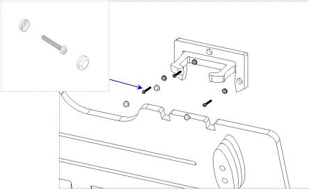
Installing Safety Seat Retaining Bracket Assembly
