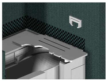
Shower Deck Safety Seat Retaining Bracket Installed. Seat In Up Position.  $28\,$
