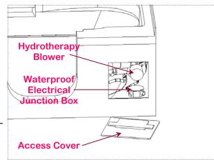
Access Cover Removed, Showing Hydrotherapy Electrical Junction
