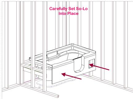
6. Set the bathtub in place and firmly press into the mortar bed. Have a level handy to check for levelness throughout this procedure. Press the bathtub into the mortar far enough so that the ledges of the bathtub rest on the framing members.
