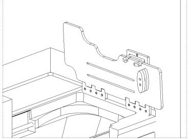
Shower Deck Safety Seat Retaining Bracket Installed. Seat In Up Position.
