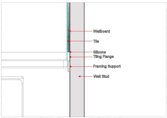
Typical Installation of Wallboarding And Tile - Section View Safety Bath So-Lo With Optional Heated Shower Deck Shown
