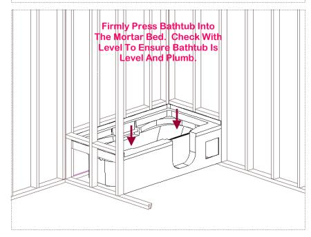
7. **DO NOT UNDER ANY CIRCUMSTANCES** nail, screw, or otherwise permanently fasten the bathtub to the wall, stud, or any other member. The bathtub will not shift or appear loose if the above steps have been followed.
