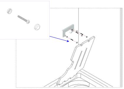
Installing Safety Seat Retaining Bracket Assembly
