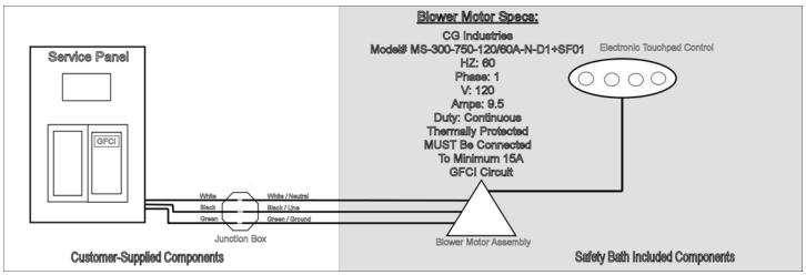
Safety Bath Warm Air Massage Hydrotherapy System Wiring Schematic (Canada & U.S.A.)
