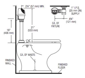
When installing the G2 Optima Plus in a handicap stall: Per the ADA Guidelines (section 604.9.4) it is recommended that the grab bars be split or shifted to the wide side of the stall. If grab bars must be present over the valve, use the Alternate ADA Installation as shown to the right.
