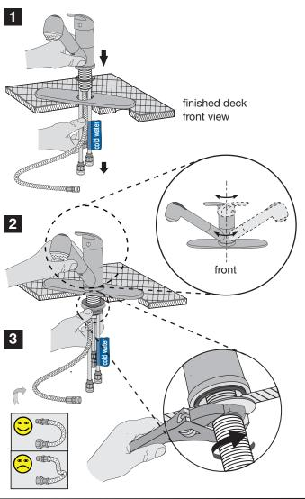
Step 3 Connect pull-out spout hose to supply
