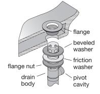
Tighten flange nut up against friction washer to evenly compress beveled washer while also ensuring flange is centered in drain opening.
