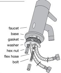
• Center faucet in sink mounting hole and tighten hex nuts.
