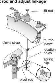
• Insert lift rod into end of clevis strap and fasten with thumb screw at
