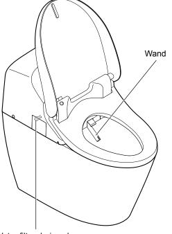
Water filter drain valve
