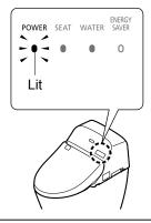
Is the ENERGY SAVER LED lit? ■ While the LED is lit, energy saver (Page 24) is in operation, so the toilet seat temperature may be reduced or the warm water heater and toilet seat heater may be turned off.
