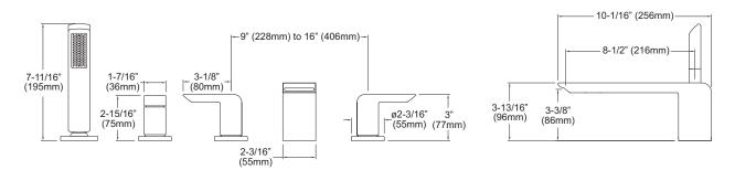
IMPORTANT NOTE: This valve/trim can only be installed in a built-up deck. It cannot be installed on pre-finished deck or on tub rim.
