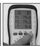
Press and hold "SEND" to log the current readings.
