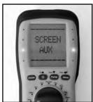
Scroll "▲"UP or "▼"DOWN Scroll "▲"UP or "▼"DOWN Scroll "▲"UP or "▼"DOWN Rotate selector to "AUX" to AUX. Press "SEND".
