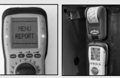
To view logged results rotate the test selector to "MENU" scroll to the "REPORT" screen and select desired test. Select "VIEW" and scroll to desired log and view results. Press "SEND" to print.
