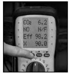
Press and Hold the "A" UP button to toggle between fuel test screens 1 and 2. Flue Test Pg.1: O2, CO, Draft (P) and TF. Flue Test Pg. 2: CO2, NO, Efficiency and Excess Air. (NO<sup>1</sup> upgrade available on Eagle 2 and 2X. NO<sup>1</sup> comes standard on Eagle 3 and 3X.)
