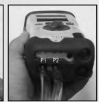
Connect true draft hose and probe into P1. Use P2 for Differential. Place probe tip in draft. You can also use the stack to measure draft. Connect static pressure hose to P1 and P2 to measure differential pressure..
