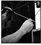
Insert Flue Probe in stack. Adjust the cone so the end of the probe is approximately. at the center of the stack (4" stack adjust cone to aprox 2" from end of probe.)
