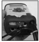
Connect flue probe thermocouple connector to T1, and connect flue probe to water trap as shown above. Use optional probe with T2 for inlet temperature.
