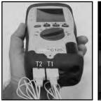
Connect flue probe thermocouple or accessory thermocouple connector to T1. Connect accessory thermocouple probe to T2. Compatible with any K-Type thermocouple probe or clamp.
