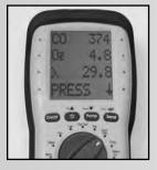
Rotate test selector to Exch Test. Call for heat on the system. Observe and wait for O2 readings to stabilize.
