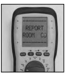
To view results rotate test selector to "MENU" and select "REPORT" Scroll to "ROOM CO" and press "SEND".
