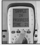
The meter will wait 30 seconds and then record the Post-Blower values for CO, O2 and Excess Air. Test results will automatically be stored to exchange reports. Report includes both Pre and Post Blower test segments.
