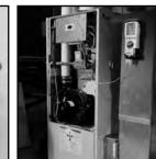
Place thermocouples in test locations to start testing.
