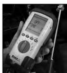
Once complete, remove probe from the stack and allow the analyzer to purge in fresh air until CO sensor readings return to ZERO and O2 reads 20~21% (20.9%). Continue to the next test or turn off your analyzer if finished. NOTE: print and store functions may be used at any point during testing.
