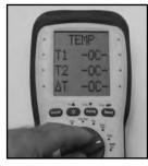
Rotate test selector to Temp
