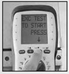
After the blower turns on press PUMP to start the Post- Blower test.
