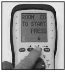
No probes or hose connections required for this test. Place handset in the area to be tested. Rotate test selector to Room CO
