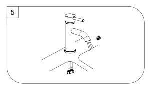
Important: After installation is completed. Turn on water supply and allow both hot and cold water to run for at least one minute each. While water is running, check for leaks.
