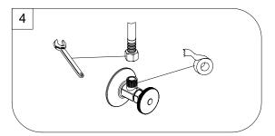
Apply pipe tape onto threads of water supplies. Use wrench when tightening the hose connection, do not overtighten.
