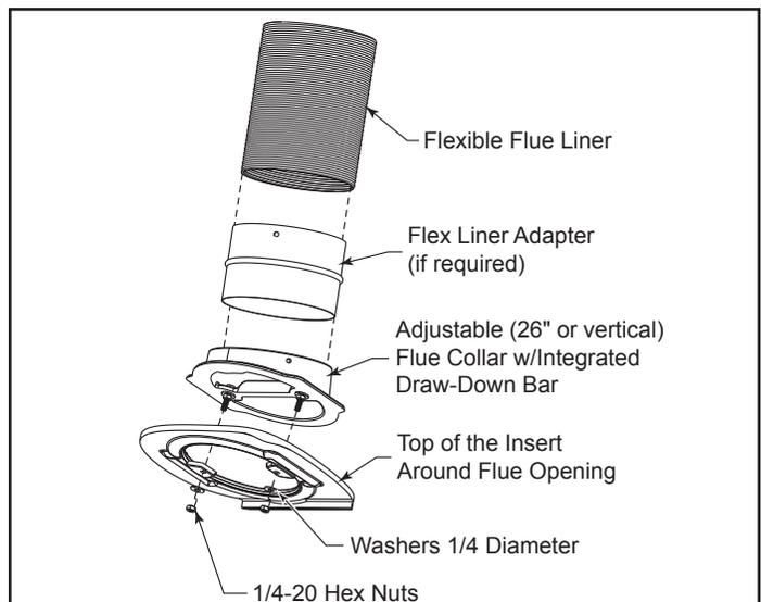
**Figure 6** - Components of the venting system.
