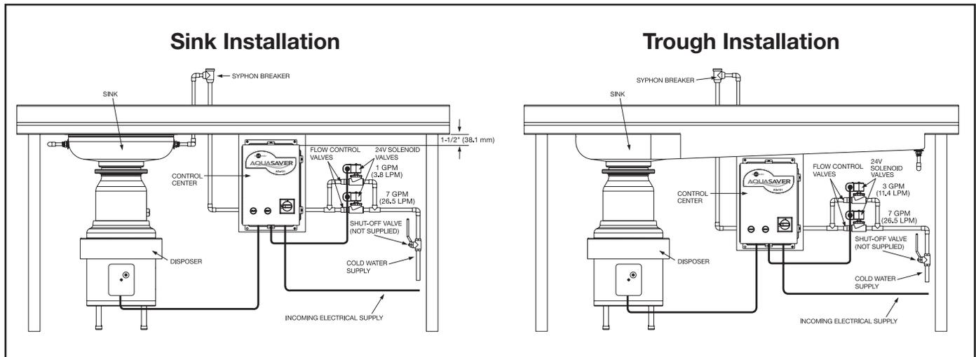
Figure 2. Typical Installation Diagram
