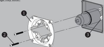
**NOTE:** Depending on the mounting depth of the Delta Valve, the Valve Mounting Plate (1) may contact either the surface of the wall, or the Plaster Guard of the Delta Valve when secured into the final position.
