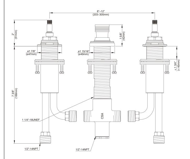
\* Installation method shown is for deck thickness of less than 1-3/4". If the installation is for deck thickness between 1-3/4" and 3-1/2", the sleeve nut needs to be reversed.
