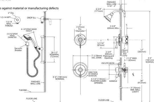
NOTE: This valve is not intended to be used as a shut-off valve. To prevent the potential of cross flow, check valves must be integral to the supply valve or installed in both hot and cold water supply lines.
