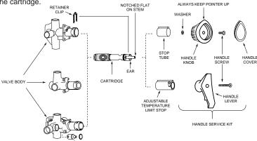
Re-insert cartridge by pushing it all the way into the body until the front of the ears on the cartridge shell are flush and aligned with the body, (see illustration). Replace the retainer clip so that the legs straddle the cartridge ears and slide down into the bottom slot in the body. This prevents the cartridge from rotating and locks it in the body. The notched flat on the stem must point UP when mounting handle, with pointer UP. Re-install stop tube, handle parts and handle knob or lever.
