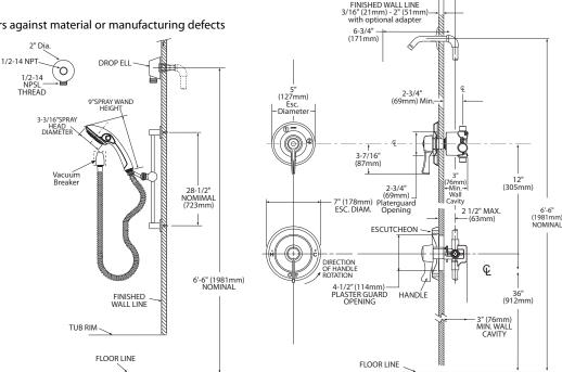
NOTE: This valve is not intended to be used as a shut-off valve. To prevent the potential of cross flow, check valves must be integral to the supply valve or installed in both hot and cold water supply lines. \*Refer to (ADAAG) guidelines or local codes for proper ADA installation.
