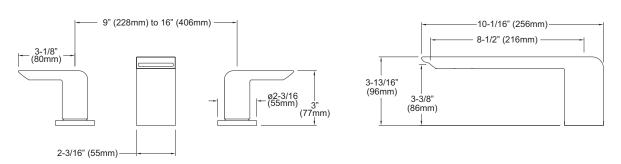
IMPORTANT NOTE: This valve/trim can only be installed in a built-up deck. It cannot be installed on pre-finished deck or on tub rim.
