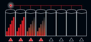
The "lead" boiler modulates with demand to capacity. As demand increases, additional boilers fire and modulate to capacity. This continues, with additional boilers firing and modulating to capacity until all units are operating. Every 24 hours, the SMART SYSTEM automatically shifts the lead boiler role to the next in the sequence, distributing lead-lag runtimes equally.
