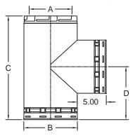
Note: Insulated Tee - 10" - 12" galvanized casing only. 14", 16", and 18" components are intended for use on chimney extensions only.
