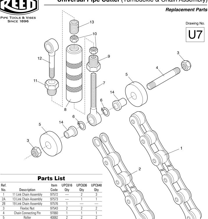
Complete Turnbuckle & Chain Assembly #97579 UPC636, UPC648 #97580 UPC616 (Item #1 not included with either)
