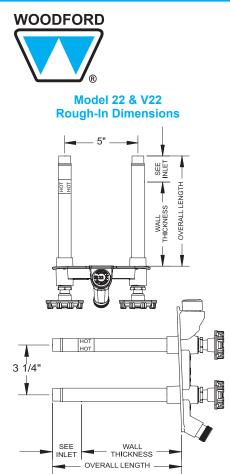
Overall Length Dimension: Add wall thickness and inlet option length shown in chart on reverse side.
