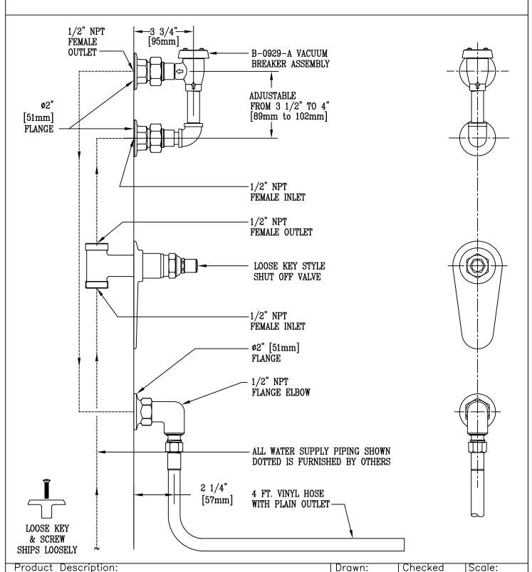
BED PAN WASHER w/ SINGLE TEMPERATURE SUPPLY, LOOSE KEY STOP, ATMOSPHERIC VACUUM BREAKER & 4 FT. VINYL HOSE w/ PLAIN END
