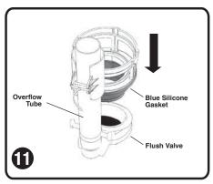
Slide Base down overflow tube, seating Blue Silicone Gasket into flush valve. Unit is designed to install vertically with both angled and straight flush valve openings.
