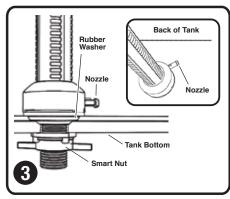
Install Valve with Rubber Washer seated as shown above. Nozzle should point back and right within tank.
