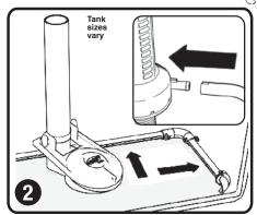
Lay J-tube along back of bottom of tank, with Sliding Elbow in back right-hand corner, as shown. Place Valve in tank to estimate J-tube length needed. Before attaching J-tube, adjust length by pulling J-tube through Sliding Elbow if needed. For small tanks, trim connecting end carefully to fit. Push J-tube onto bottom port of valve.
