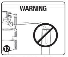
NOTE: Refill Tube must be positioned above overflow tube.
