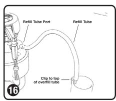
Install Refill Tube of fill valve. Attach Clip to overflow tube. Trim tubing to size to prevent kinking and install tubing ontothe Mini-Valve Refill Tube Port.
