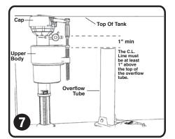
Adjust Valve height so that top of Cap is even with top of tank. This height should allow the final Float adjustment to be achieved with Thumb Screw (described later). Turn Upper Body counterclockwise to lock in Valve height.
