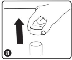
If overflow tube has a cap, remove it and discard before installing Refill Tube. Proceed to installing the dual flush converter.
