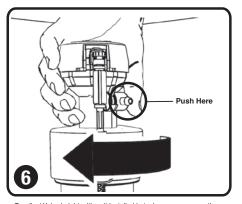
To adjust Valve height with unit installed in tank, grasp upper portion, placing thumb on gray side of Mini-Valve and push clockwise  $\frac{1}{4}$  turn. Slide Upper Body to adjust up or down.
