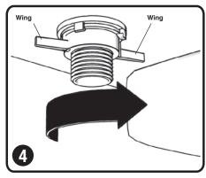
The Smart Nut should only be hand tightened and should make 1-3 audible clicks to signal it is tight. Wings are designed to bend if Smart Nut is overtightened, preventing leaks and cracking.
