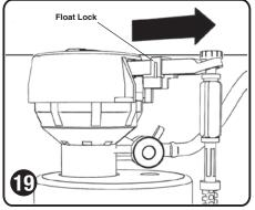
Turn on water and when water is clear, disengage Float Lock to fill tank. This willprevent debris from plugging up Valve.
