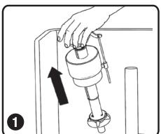
Shut off water, flush toilet to empty tank and remove old toilet fill valve.
