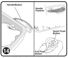
For units with Handle, position and hand tighten Handle in a standard operating position.
