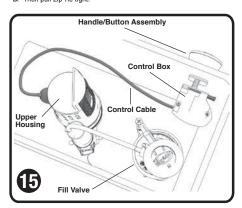
Match the color-coded hole to the corresponding Handle/Button connection pieces, attach white Control Box to Handle/Button, Audible click assures that Clip has secured Control Box to Handle/Button and unit will no longer pull apart without pushing the Green or Blue Push Release.
