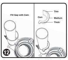
If gap appears around overflow tube, estimate width of space and use with thick, medium or thin section of Cam, as needed to fill gap.
