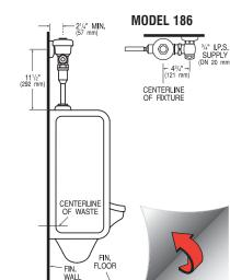
When mounted on an ADA accessible bowl, the rough-in to the supply inlet should be no higher
