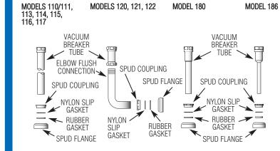
(B) Insert Tube into Fixture Spud.
