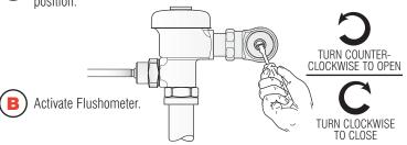
( C ) Adjust Control Stop after each flush until the rate of flow delivered properly cleanses the fixture.
