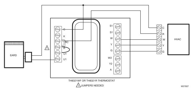
Fig. 4. Typical M847D-VENT wiring.
