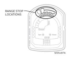
Fig. 5. Air Flow Adjustment.
