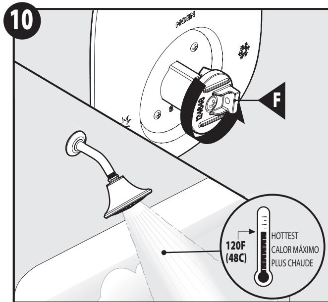
Turn Handle Adapter (F) towards hot side to test hot water temperature.
