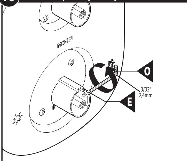
Retighten Stop Tube Screw (**E**) with 3/32" Hex Key (**O**).
