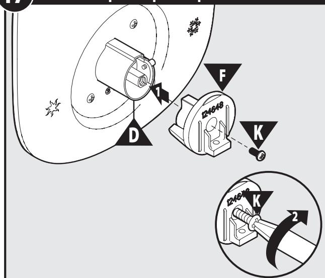
1. Re-Install Handle Adapter (F) and Handle Adapter Screw (K) onto lower Stop Tube (D).
