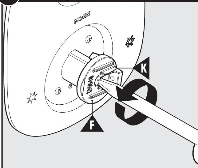
Loosen Handle Adapter Screw (**K**) with a Philips Screwdriver.
