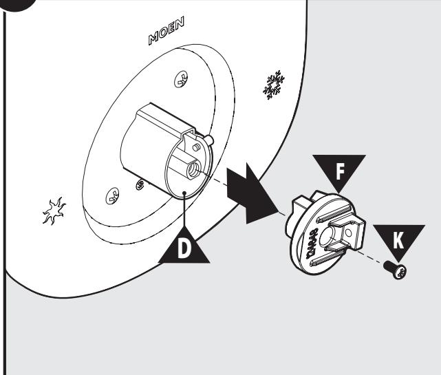
Remove both Handle Adapter Screw (**K**) and Handle Adapter (**F**) from lower Stop Tube (**D**). Set aside for re-installation once temperature adjustment is complete.
