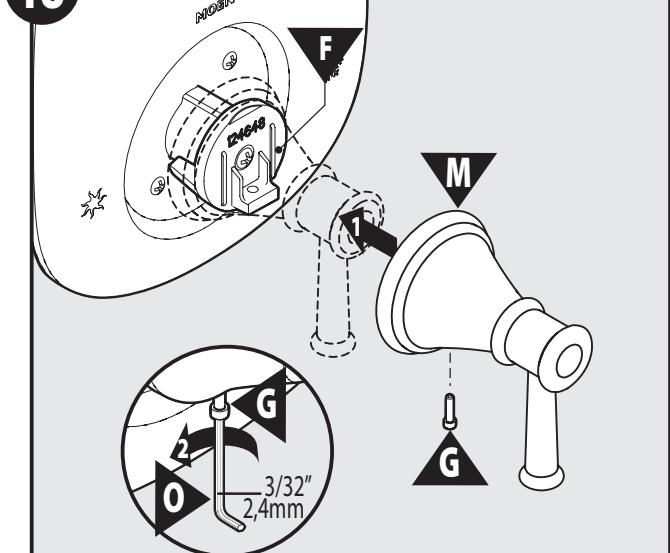
1. Install Lever Handle (M) onto Handle Adapter (F). Also, install Set Screw (G) into bottom of Lever Handle.
