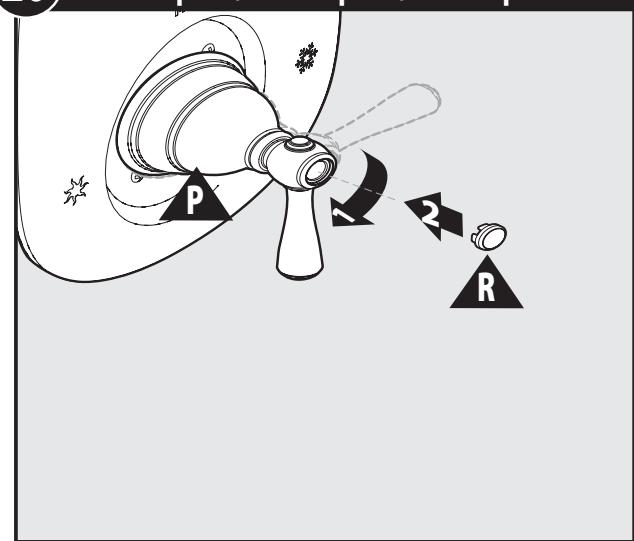
1. Rotate Lever Handle (P) 90° clockwise as shown.
