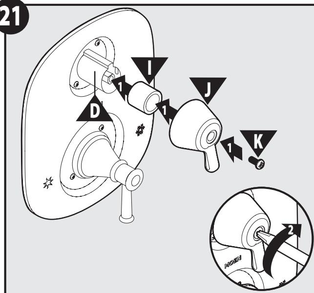
1. Install Spacer (I), Lever Handle (J), and Handle Adapter Screw (K) onto upper Stop Tube (D) in order as shown.
