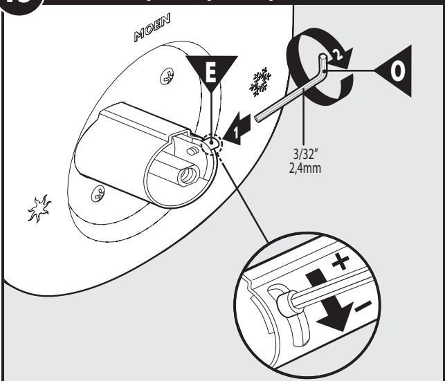
1. Insert 3/32" Hex Key (**O**) into Stop Tube Screw (**E**).
