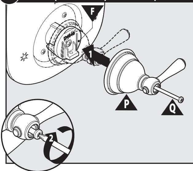
1. Install Lever Handle (P) onto Handle Adapter (F). Also, install Handle Screw (Q) into handle and handle adapter.
