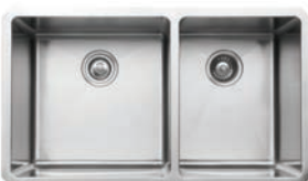
KHU103-33 ..... 33 inch Undermount 60/40 Double Bowl 16 Gauge Stainless Steel (L) 32 3/4" x (W) 19" x (D) 10" Minimum Cabinet Size: 36" Included: grids KBG-103-33-1 & KBG-103-33-2, strainers BST-1 & ST-1
