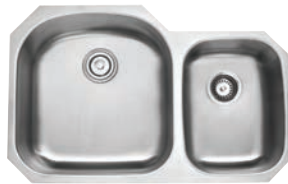
KBU23 ..... 32 inch Undermount 60/40 Double Bowl 16 Gauge Stainless Steel (L) 32 3/8" x (W) 20 1/2" x (D) 9" Minimum Cabinet Size: 36" Included: grids KBG-23-1 & KBG-23-2, strainers BST-1 & ST-1
