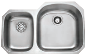
KBU25 ..... 32 inch Undermount 60/40 Double Bowl 16 Gauge Stainless Steel (L) 32 3/8" x (W) 20 1/2" x (D) 9" Minimum Cabinet Size: 36" Included: grids KBG-25-1 & KBG-25-2, strainers BST-1 & ST-1
