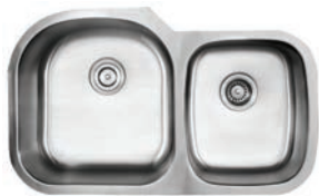
KBU27 ..... 35 inch Undermount 60/40 Double Bowl 16 Gauge Stainless Steel (L) 34 3/8" x (W) 20 1/2" x (D) 9" Minimum Cabinet Size: 39" Included: grids KBG-27-1 & KBG-27-2, strainers BST-1 & ST-1
