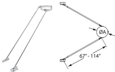
Use to support the chimney when it extends more than 4' above the roof. Provides stability to chimney against wind and snow. Mounting brackets and adjustable legs included.
