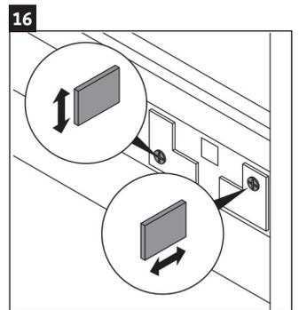
Level the vanity drawer by adjusting the two screws.
