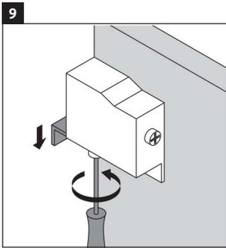
Using the crewdriver adjust the vanity mounting hinge system counter-clockwise.
