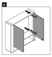
Remove the mirror fronts of the cabinet by unlatching each hinge.
