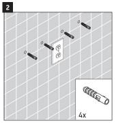
Drill the anchor holes that have been marked.
