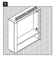
Check the cabinet is leveled and securely attached to the wall.
