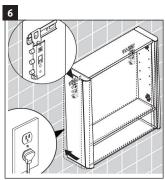
Plug the unit into outlet and lift the unit up and onto the mounting brackets.
