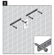
Screw the bracket(s) to the wall the specified locations. For wood stud walls, bolts should be screwed into wood backing.
