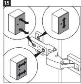
The top screw will adjust up and down. Back screw will adjust closer and further. From the mirror cabinet and front screw will adjust left and right.
