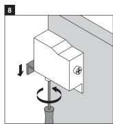
Using the screwdriver, adjust the vanity mounting hinge system counter-clockwise.
