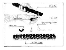
Install the cutter chain around this assembly (chain bar and sharpening holder assembly). Push the bent portion of the sharpening holder to maintain the tension on the cutter chain and tighten the wing nut securely.
