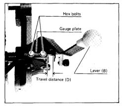
7 mm (9/32"). Tighten the hex bolts to secure the gauge plate. Cut the first hole with the lever (B) pushed away from you. Then pull the lever (B) toward you and cut again to enlarge the hole.
