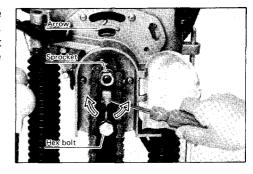
Turn the adjusting screw to increase the tension on the cutter chain. Pull the middle of the cutter chain lightly. When there is a clearance of approx.  $5-6 \text{ mm } (3/16^{\prime\prime}-1/4^{\prime\prime})$  between the chain bar and the cutter chain, the tension on the cutter chain is adequate.
