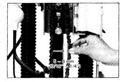
After adjusting the tension, tighten the hex bolt firmly to secure the chain bar. Additionally tighen slightly the adjusting screw. Close the chain cover.
