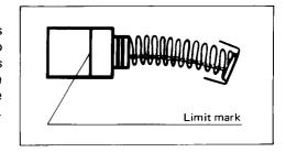
Use a screwdriver to remove the brush holder caps. Take out the worn carbon brushes, insert the new ones and secure the brush holder caps.
