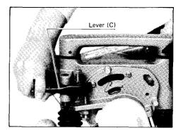
Loosen the hex nut securing the adjusting hex bolt. Turn the adjusting hex bolt until the cutter chain reaches the desired position, then tighten the hex nut.
