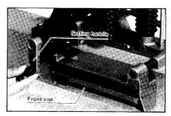
Turn the setting handle until the front edge of the yellow indicator plate is aligned with the cutting line (B).
