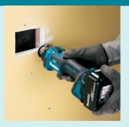
High power Brushless motor with 32,000 rpm for rapid cutting
