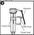
Pull the adjusting rod, and raise or lower the flxed ring to the desired water level.
