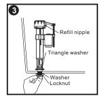
Unscrew the locknut and washer. Position the fill valve into the tank, then screw the washer and locknut. (Torque  $3\sim4N^*m$ )
