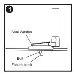
Unscrew the fixture block, Put the flush valve into the tank flush hole, and make sure the fixture block is put into the tank...
