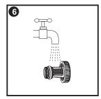
Clean the filter net, then put it back to the filter body.
