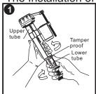
Take off the tamper proof, and adjust the beight by screwing the upper and lower tube. Then fix the tamper proof.
