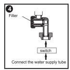
Connect one side of soft tube to the filter and the other side to the fill valve. And then connect the switch and water supply tube.
