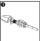
Take off nut and gaskets,install rod through tank hole.then put on gaskets and tighten nut,just follop pirture
