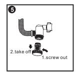
Turn off the switch and take out the filter net.
