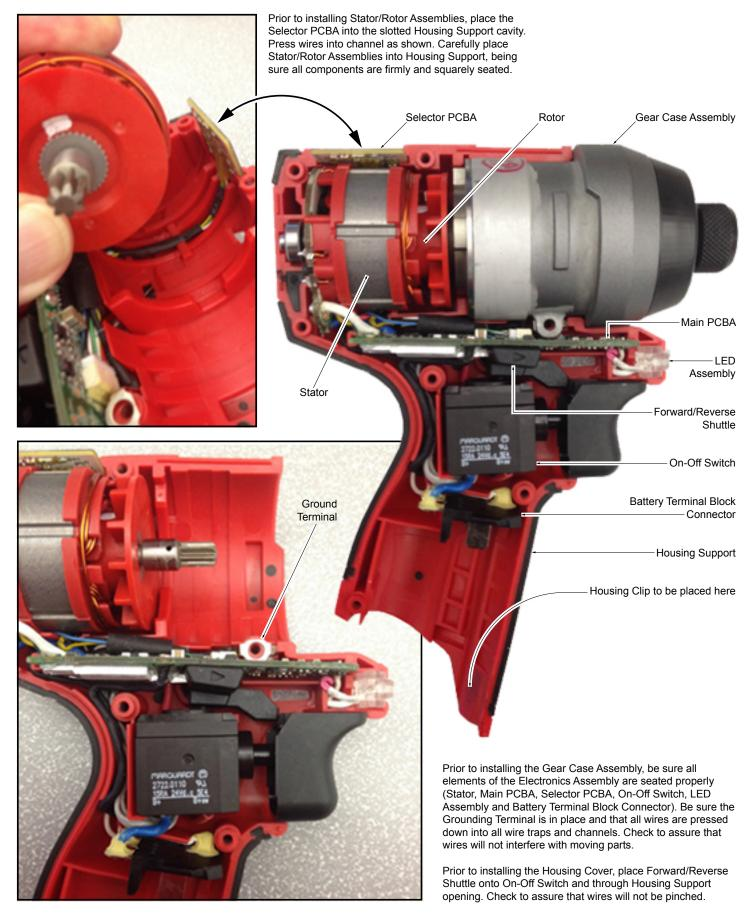
Secure the Housing Cover to the Housing Support with seven M3 x 16mm ST T-10 Screws. Be sure to replace the Housing Clip at the bottom of the battery opening.
