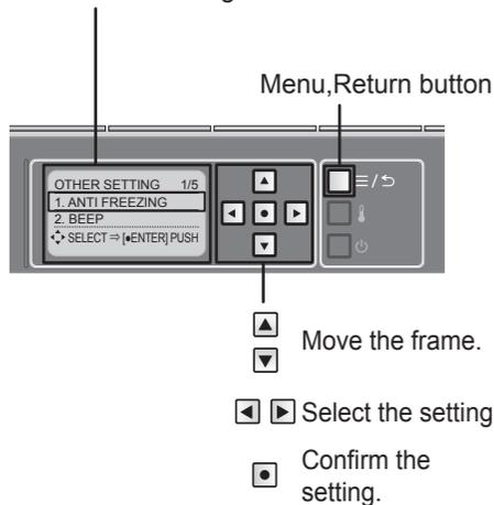
Set whether or not to run the water for the bowl unit and top unit automatically at a fixed interval in order to prevent freezing
