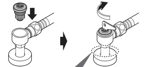
Hold the pipe with hands while tightening the cap.
