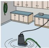
Draining waterbeds, hot water tanks, appliances, aquariums, and other emergency dewatering needs Models: MPFVK115, MPFV12, MPDP, MPTC
